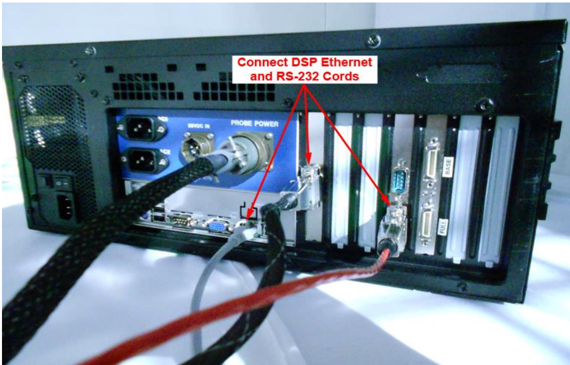
Figure 2.2.5 Connecting the DSP to the Data Acquisition System
