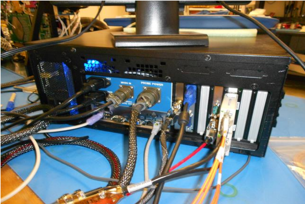
Figure 2.4.1: 3V-CPI Data Acquisition System with all cables connected
