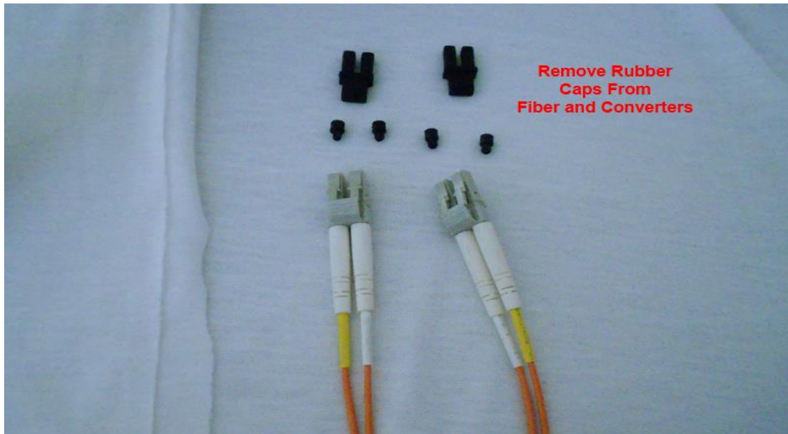
Figure 2.2.9 Removing caps from Fiber Cables and Converters
