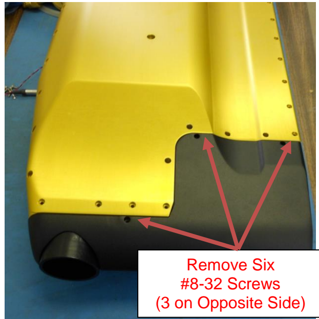
Figure 6.4.1: Screw locations for fairing removal required for purging
